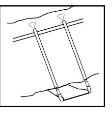
**STEP 9:** When attaching the pool wall insulation, you will need to start about 4 inches from the plumbing openings. So that when you are finished with the insulation, there should be about an 8 inch gap exposing the two plumbing openings.
