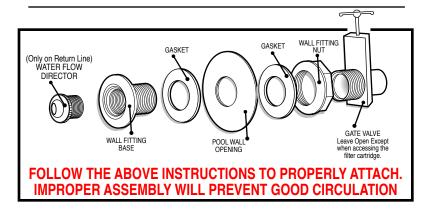
**IMPORTANT NOTE:** When operating your pump and heater, the Gate Valves should be left open. When accessing your cartridge filter for cleaning, they should be blocked. It is a common mistake to start your pump and heater and the Gate Valves are closed. The heater will not turn on in this case.
